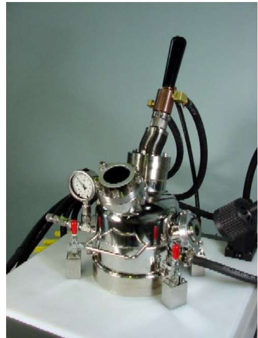
Bell jar chamber in closed position. Observe the view port with eye protection shield, illumination port and the stinger with bellows and handle.
