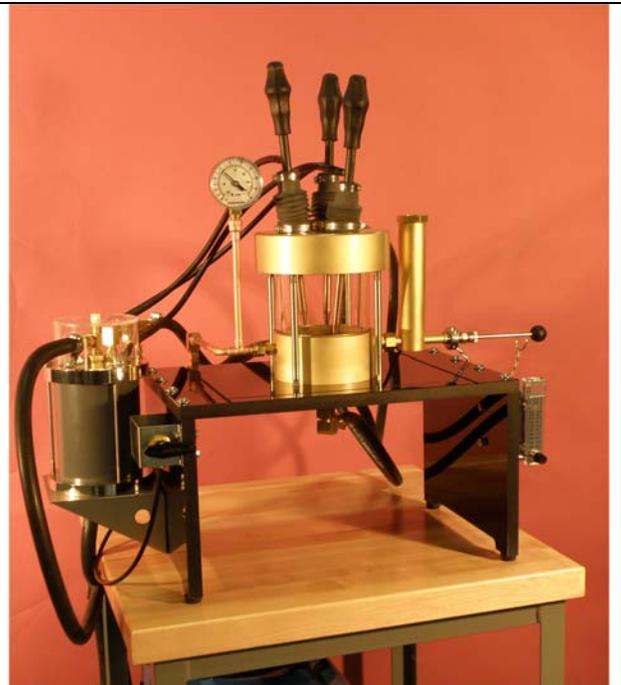
*Tri-arc chamber with gas and vacuum system and optional load lock. The welding glasses have been removed for visibility.*
