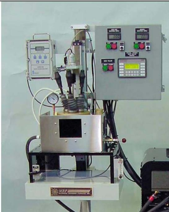
*Tri-Arc melt chamber with optional crystal growing kit, rotating hearth, load lock, and oxygen monitor.*
